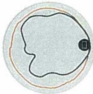
Figure 3. T310d 5GHz Azimuth Antenna Patterns
